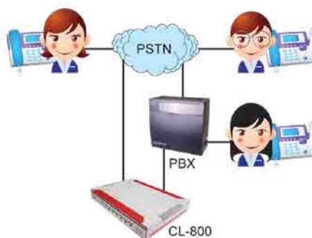
By default the organizer uses the 0-9, \* and # buttons of a touch-tone phone to manage the conference room and meeting activity. If optional Discuss (computer software) and N-port (a small hardware enabling connection between CL-800s and computer) are installed, the organizer can instead use computer keyboard and mouse to manage the room and activity.
